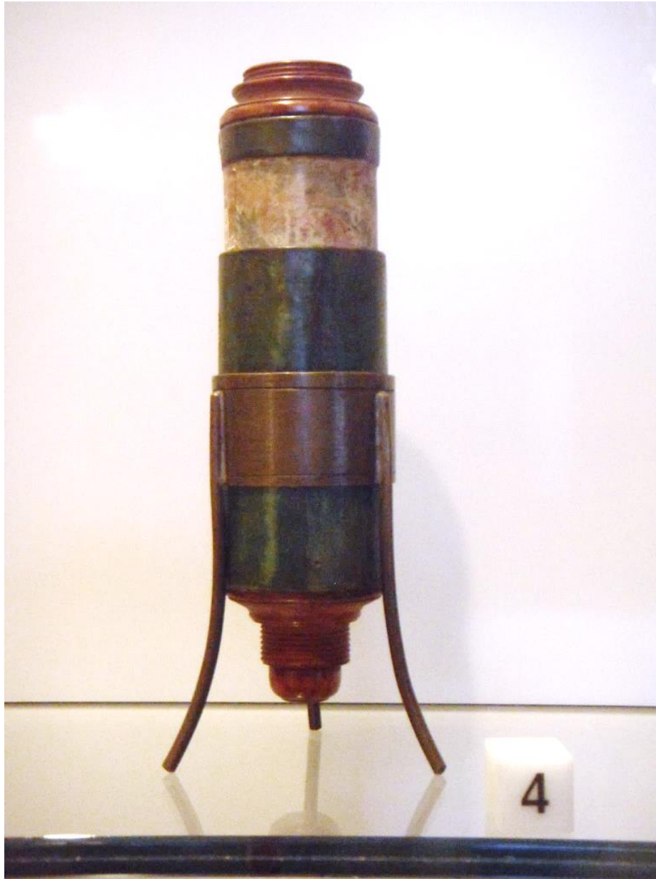
Figure 4. An example of a seventeenth century Galilean compound microscope, credited to optician Giuseppe Gampani (1635 – 1715) [Museo Galileo, Florence, inv. no. 3429 – Photo J. Servello].
