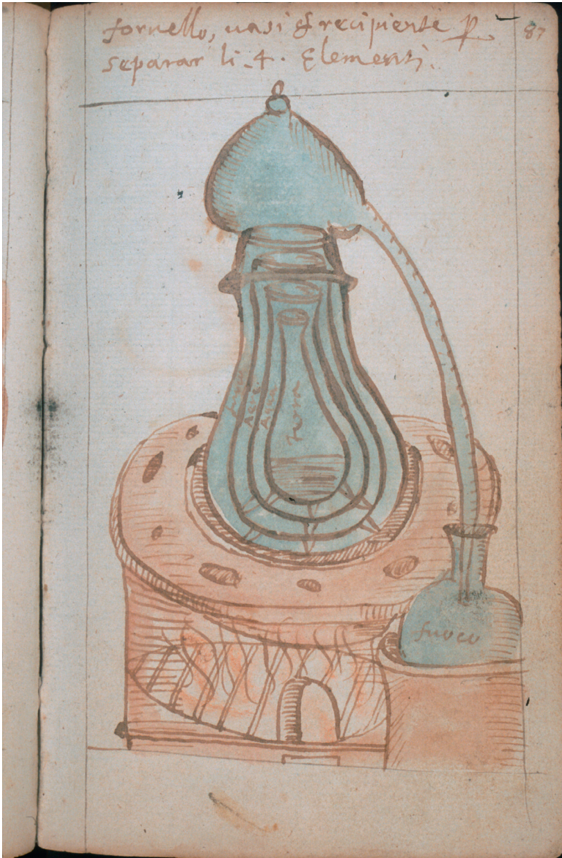
Figure 1. Small furnace for the simultaneous separation of the four elements where earth, water, air and fire are arranged in suitable vessels, inserted into each other. Antonio Neri, MS Ferguson 67 (1598-1599), f. 87r. Glasgow University Library, Special Collections.
