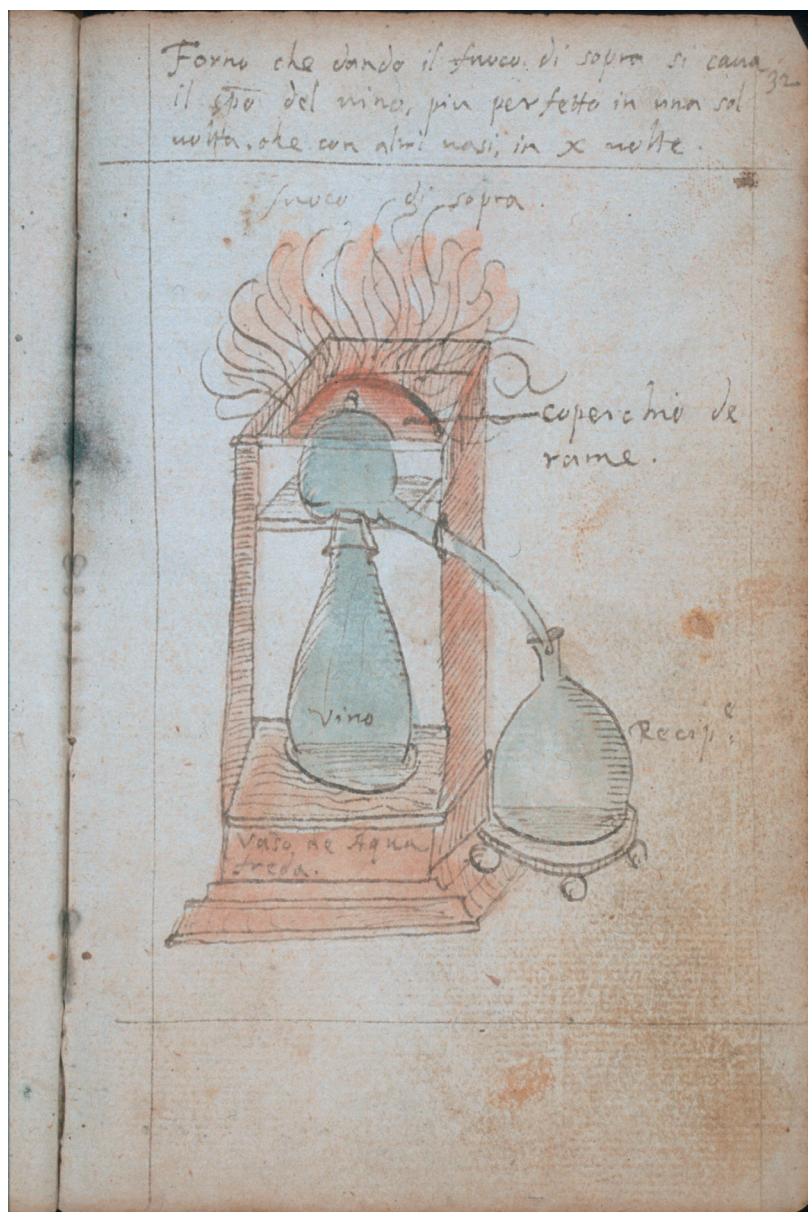
Figure 4. Furnace for the distillation of wine, characterized by the particular position of the fire which is not in contact with the container, but is placed at the top, above a copper lid. Neri, Ferguson (cit. Fig. 1), f. 32r. Glasgow University Library, Special Collections.
