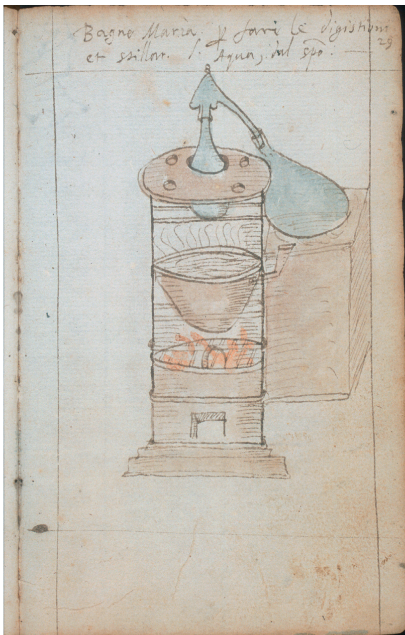
Figure 3. Furnace used for the Bain Marie, a system for heating and distillation used to treat particularly delicate substances, that would deteriorate if subjected to a direct flame. Neri, Ferguson (cit. Fig. 1), f. 29r. Glasgow University Library, Special Collections.
