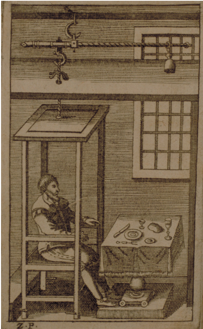
Figure 9. The scale invented by Santorio Santorio to weigh the loss of fluids during transpiration, in an engraving of 1710.
